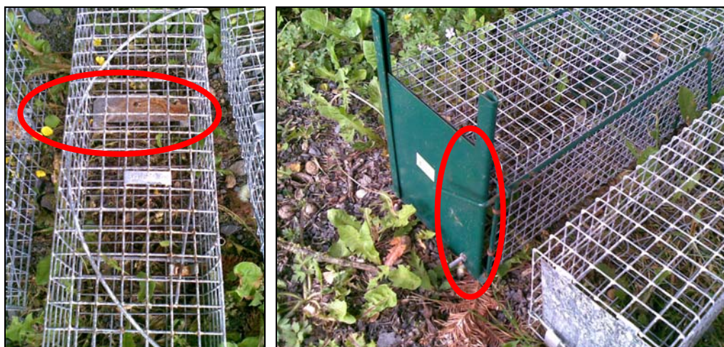
Figure 6.9 - Results of accelerated rusting tests (significant corrosion highlighted)
