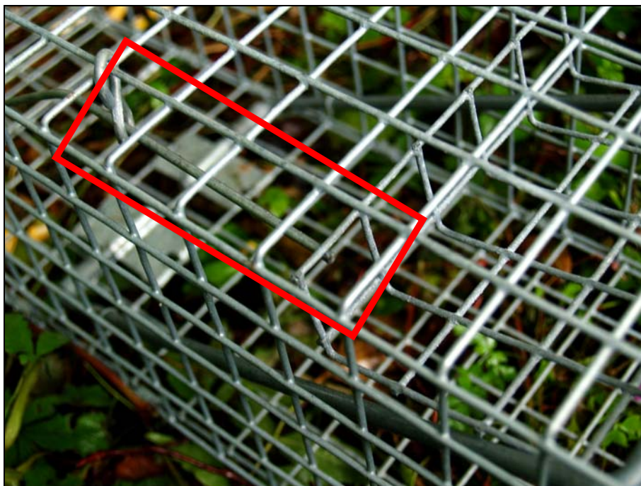
Figure 9.7 – Trap setting mechanism, with trigger highlighted
